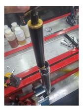
The compression side is similar to the rebound however we'll be replacing the entire tower so there's no grinding involved.
