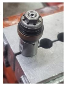
Using a 14mm spanner remove the compression tower. It may help to use some heat to break the thread lock they come installed with.
