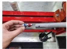
Step 8: Now using the cartridge tool remove the seal case from the cartridge, so you can remove the entire rod and piston assembly.
