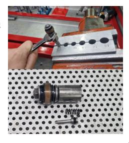
Step 7: Install the new needle and spring with a bit of grease.
