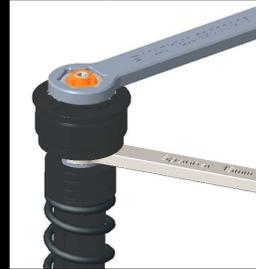
Remove the wrench 15mm by pushing the spring down again. The spring can be removed. Re-fitting is the same procedure.
