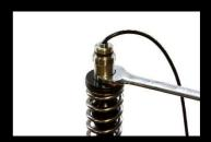
Make sure the parts ae tightened with 30Nm torque.
