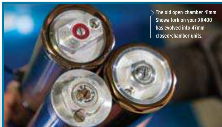
➤ WP's 43 and 48mm open-chamber forks remain, while the 48mm closed-chamber fork is fitted to MX models.
