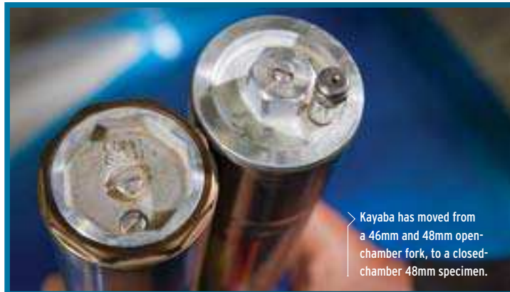
➤ The old open-chamber 41mm Showa fork on your XR400 has evolved into 47mm closed-chamber units.
