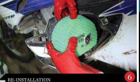
W ith the filter cleaned and oiled, reinstall the filter on its plastic frame. It's a good idea to leave the oil to set for a few hours before re-installing on the bike. Now put a generous layer of grease around the airbox seat and the sealing surface of the filter. This will prevent any dust entering around the filter. Ensure the filter is seated neatly and fastened.
