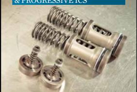
Showa and Kavaba twin-chamber forks have gained popularity but they are sometimes criticised for being harsh on small bumps. Progressive Inner Chamber Springs (ICS) are available to add position sensitivity to the normally speed-sensitive nature of dampening. So where the fork might have a standard 1.8kg/mm ICS, you can replace it with
