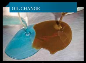
The dampening character of your suspension relies on oil for lubrication and as a medium to hold contaminants (and dirt). This stops orifices from being blocked, and prevents wear from occurring too quickly. Oil is also used for cooling. So by simply renewing the fluid, you will get the full benefit of the technology in your suspension. While doing this, seals, bearings,
