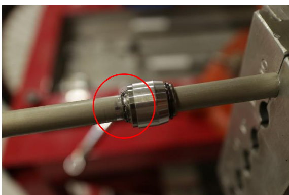
Cut the peened side until the retainer releases from the circlip
