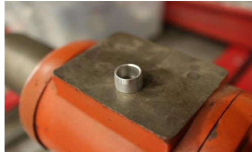
Remove the circlip and remove the bottoming cone
