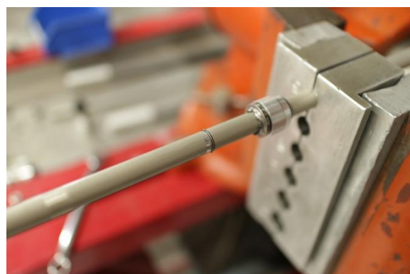
The retainer should be free from the circlip, allowing you to remove the circlip from the shaft
