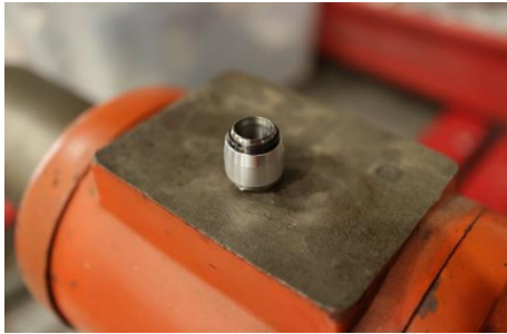
Remove the circlip and remove the bottoming cone
