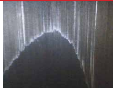
Above: The internet had a meltdown over AT upper fork tubes wearing off the anodising. It's not as widespread as the rumour mill would have it, but it happens.
